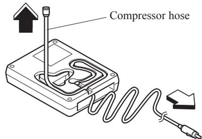
17. Install the air compressor hose to the tire valve.
