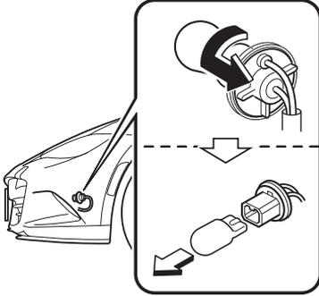
6. Install the new bulb in the reverse order of the removal procedure.
