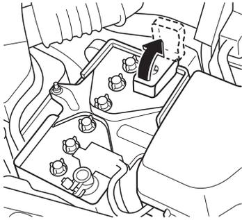
2. Make sure the booster battery is 12 V and that its negative terminal is grounded.
