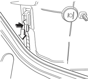
4. Pull the center of each plastic retainer and remove the retainers, and then partially peel back the trunk side trim.
