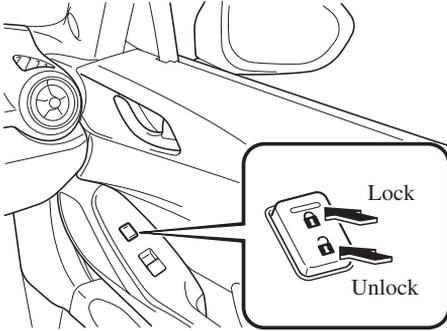
To lock both the doors and the fuel-filler lid from an open door, press the lock side of the door lock switch and then close the door.
