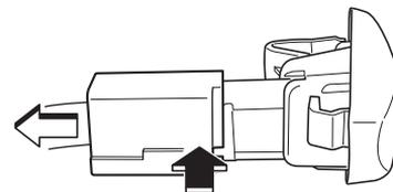
6. Install the new side turn signal unit in the reverse order of the removal procedure.
