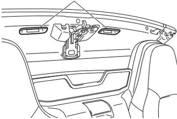
5. Sitting in a seat, grasp the convertible top's handles, and press the convertible top against the windshield. Make sure the striker engages with the anchor, move the top latch slowly, and then push the top latch upward until a latch sound is heard.
