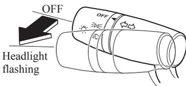
The headlight high-beam indicator light in the instrument cluster illuminates simultaneously. The lever will return to the normal position when released.
