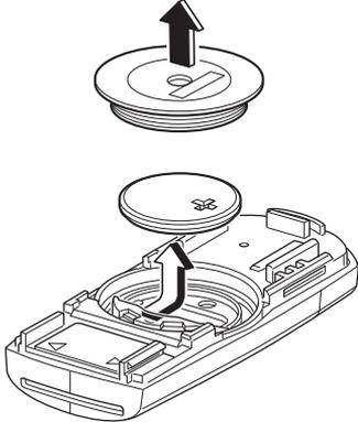
6. Insert a new battery with the positive pole facing up, and then cover the battery with the battery cap.
