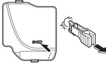
4. Inspect the fuse and replace it if it is blown.
