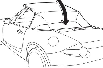
8. With the back end of the convertible top pressed, press the front end until a latch sound is heard. Lightly rock the retracted convertible top to make sure it is securely locked.
