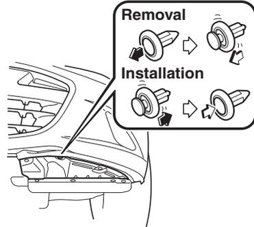
3. Turn the screw counterclockwise and remove it, and then partially peel back the mudguard.
