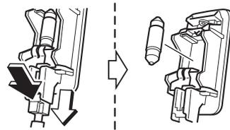
4. Install the new bulb in the reverse order of the removal procedure.
