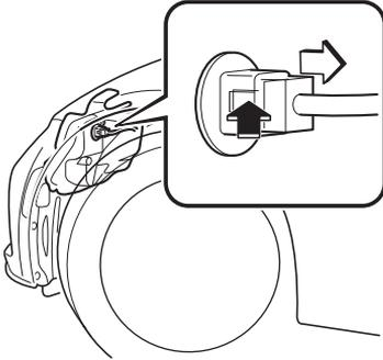
5. Turn the socket and bulb assembly counterclockwise and remove it.
