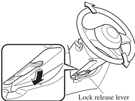
2. Tilt the steering wheel to the desired positions, then push the lever up to lock the column.
