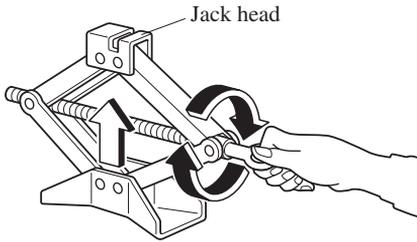
4. Place the jack under the jack-up position closest to the tire being changed with the jack head squarely under the jack-up point.
