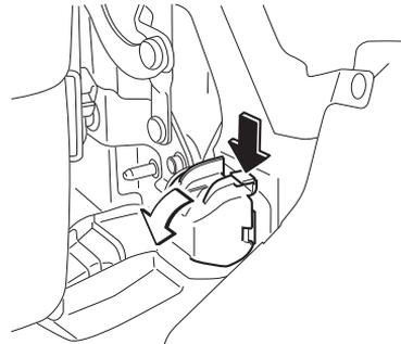
3. Remove leaves and other matter accumulated in the drain filter.
