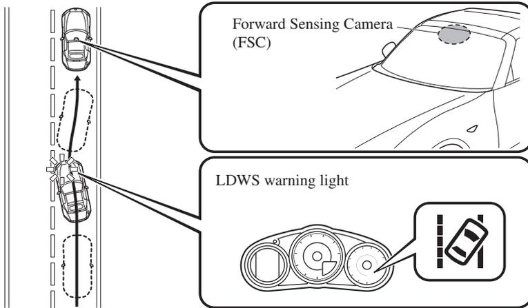
The warning light illuminates when the system has a malfunction. Refer to Warning Lights on page 4-16.
