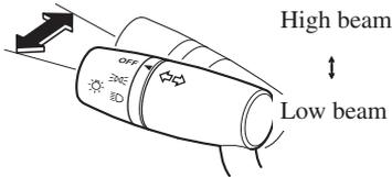
When the headlight high-beams are on, the headlight high-beam indicator light is turned on.
