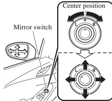
After adjusting the mirror, lock the control by rotating the switch in the center position.
