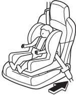
3. Place the child-restraint system on the seat without putting your weight on the seat and secure the child-restraint system with the lap portion of the lap/shoulder belt. See the manufacturer's instructions on the child-restraint system for belt routing instructions.
