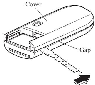
4. Twist the flathead screwdriver in the direction of the arrow and remove the cover.
