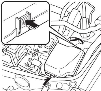
3. Remove the cover while lifting it and sliding it to the rear.
