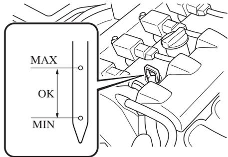
5. Pull it out again and examine the level. The level is normal if it is between the MIN and MAX marks. If it is near or below MIN, add enough oil to bring the level to MAX.
