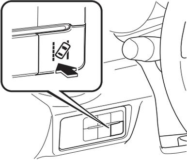
2. Drive the vehicle in the center of the driving lane while the LDWS OFF indicator light is turned off. The system becomes operational when all of the following conditions are met.
