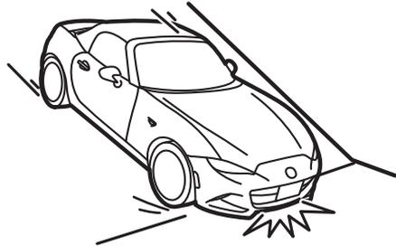
This vehicle is equipped with low profile tires allowing class-leading performance and handling. As a result, the sidewall of the tires are very thin and the tires and wheels can be damaged if driven through potholes or on rough/uneven roads at excessive speeds. Use care and reduce speed when traveling on rough/uneven roads or through potholes.
