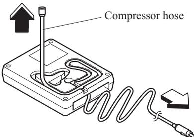
8. Install the air compressor hose which was pulled out of the air compressor to the injection valve of the bottle.
