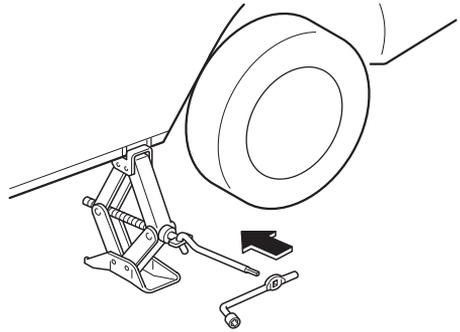
7. Turn the jack handle clockwise and raise the vehicle high enough so that the tire is raised off the ground and can be removed. Before removing the lug nuts, make sure your Mazda is firmly in position and that it cannot slip or move.
