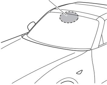
The Forward Sensing Camera (FSC) determines the conditions ahead of the vehicle while traveling at night and detects traffic lanes. The distance in which the Forward Sensing Camera (FSC) can detect objects varies depending on the surrounding conditions.
