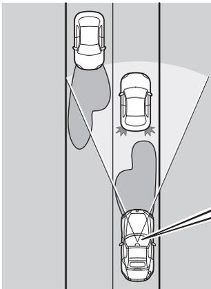
The recognition distance of the Forward Sensing Camera (FSC) varies according to the surrounding conditions.
