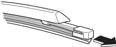
5. Remove the metal stiffeners from each blade rubber and install them in the new blade.
