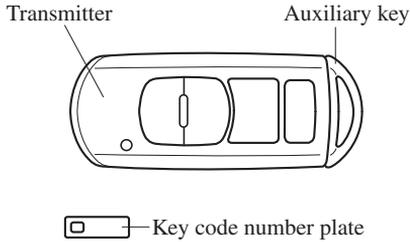
To use the auxiliary key, pull out the auxiliary key from the transmitter while pressing the knob.
