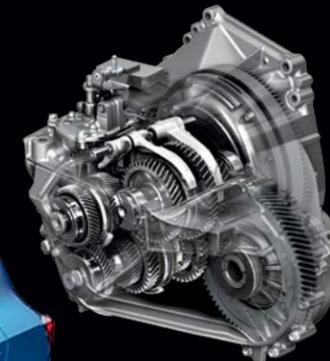
We imagined a manual transmission that helps maximize fuel efficiency more than any of its predecessors, built with less material but just as rigid. A transmission that's smaller, lighter, stronger and has the shortest shift throw in its class.
